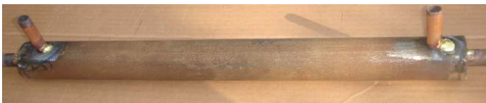
Fig. 2.1 Fabricated model of a basic heat exchanger
